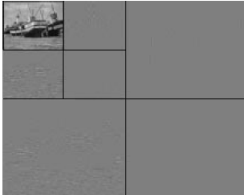
Figure G.5 – Decomposition of the EBU “Boats” picture into 7 wavelet frequency bands
