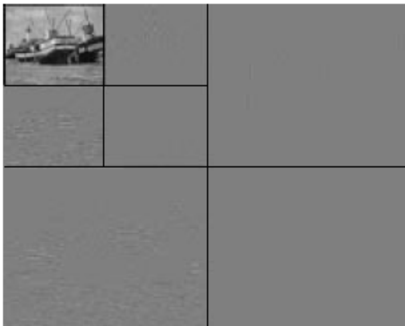
Figure F.5 –Decomposition of the EBU “Boats” picture into 7 wavelet frequency bands
