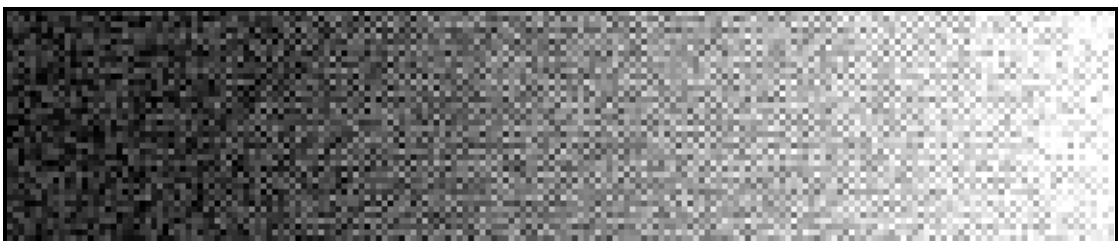
Figure A.4 – Quantized ramp with dither and random data in LSBs
