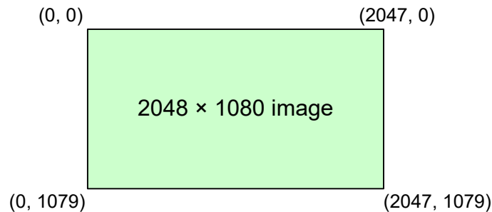
Figure 1 — Horizontal and vertical pixel numbering of 2048 × 1080 progressive images
