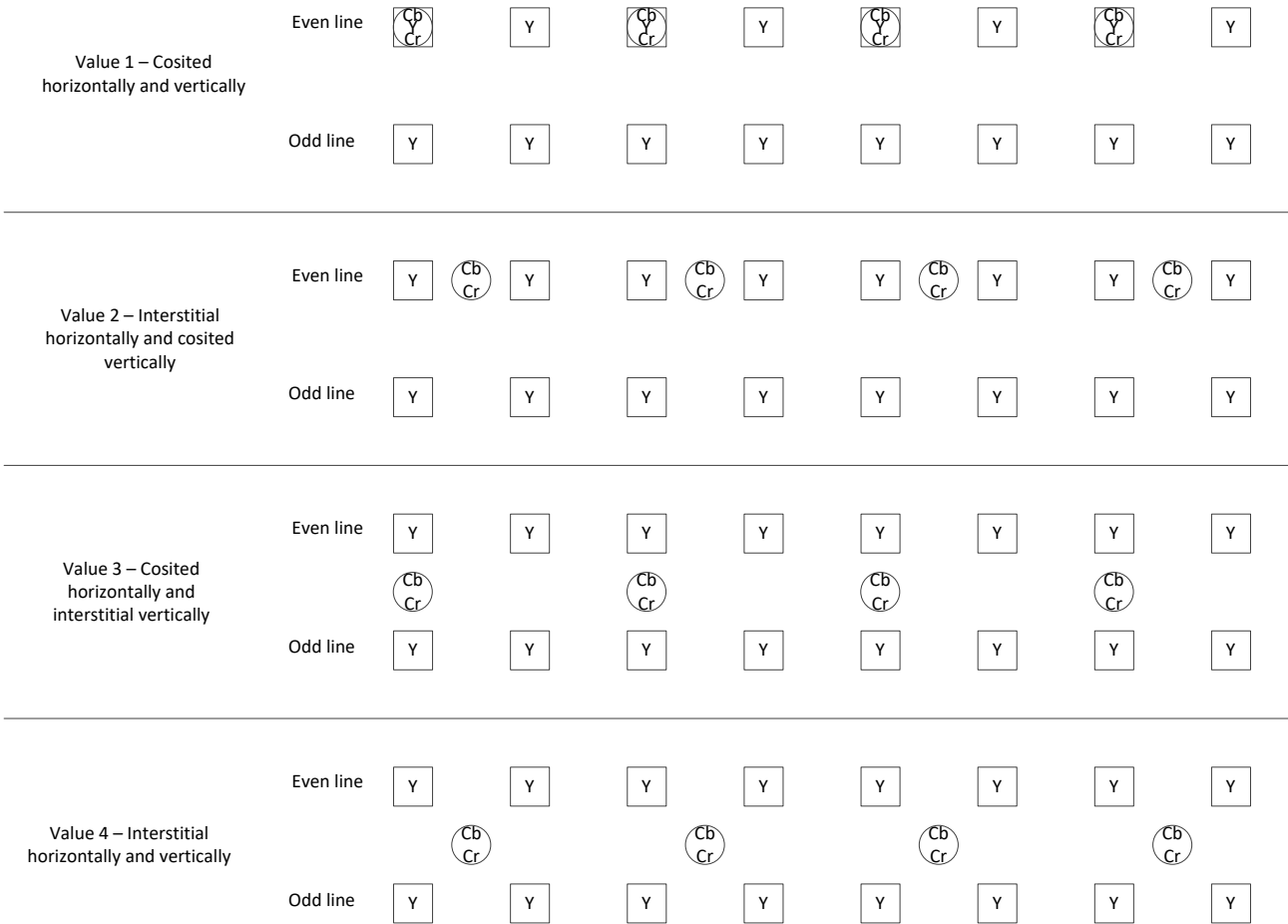
Figure 2 — Relative luminance and color difference sample positions for values of color-difference subsampling siting bits for 4:2:0 image elements
