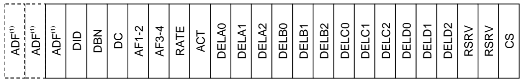
Figure 4 – Audio control packet structure
