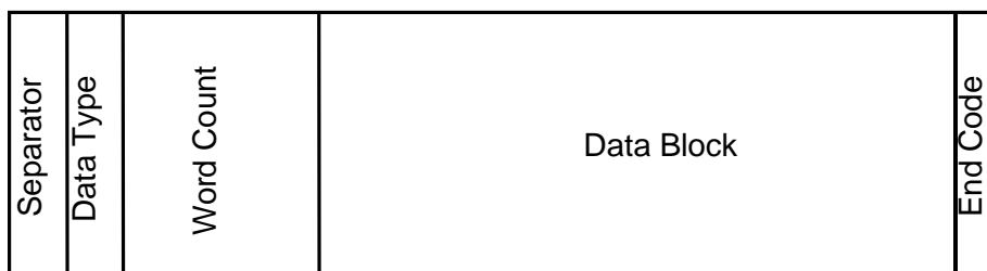
Figure 11 – Data structure (variable block size)
