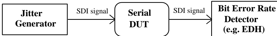
Figure 10 – Jitter tolerance measurement
