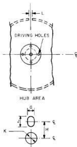
Figure 4 – Enlargement of spindle and driving hole
