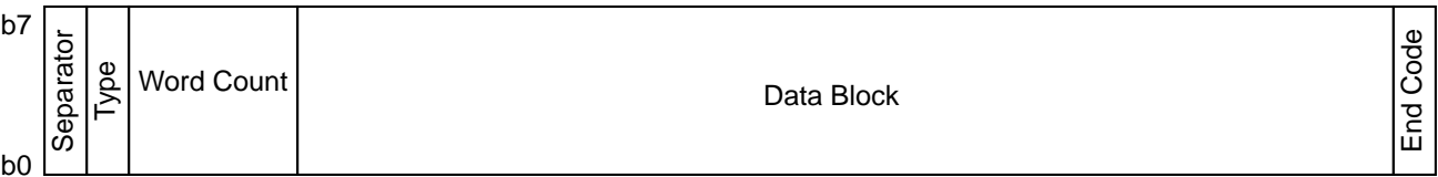
Figure 1 – Format of the SDTI variable block
