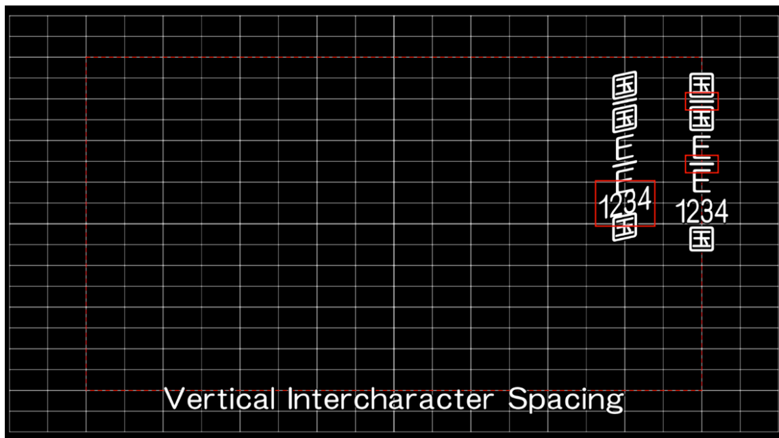
Figure 18 — Undesired vertical text intercharacter spacing sample
